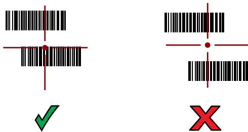
Figure 17 RS5100 Pick List Mode with Multiple Barcodes in Aiming Pattern
