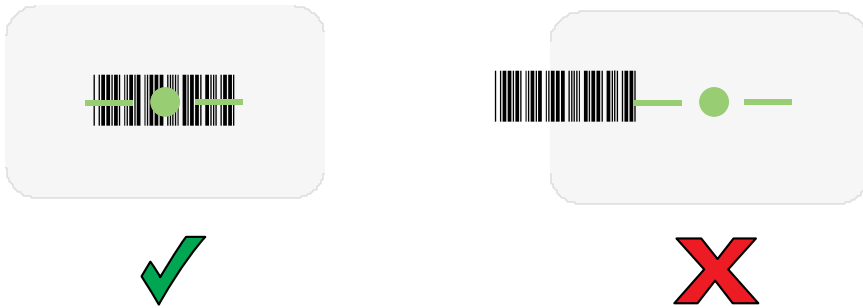
Figure 10 SE4720 Aiming for Pick List Mode with Multiple Barcodes
