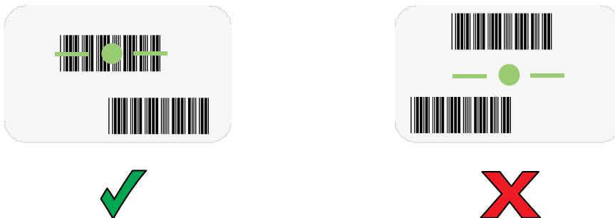
Figure 11 SE55 Aiming for Pick List Mode with Multiple Barcodes
