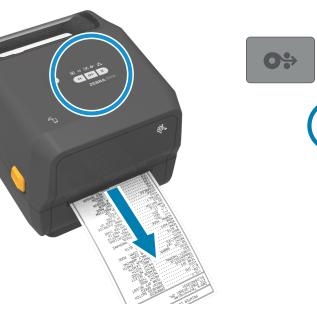
Press and hold the Feed and Cancel buttons for two seconds to print a configuration report.
