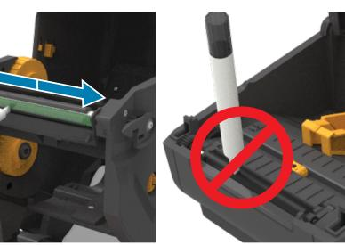
Clean printhead with cleaning pen starting from the middle to sliding to the outside. Do not use a cleaning pen on the platen.
