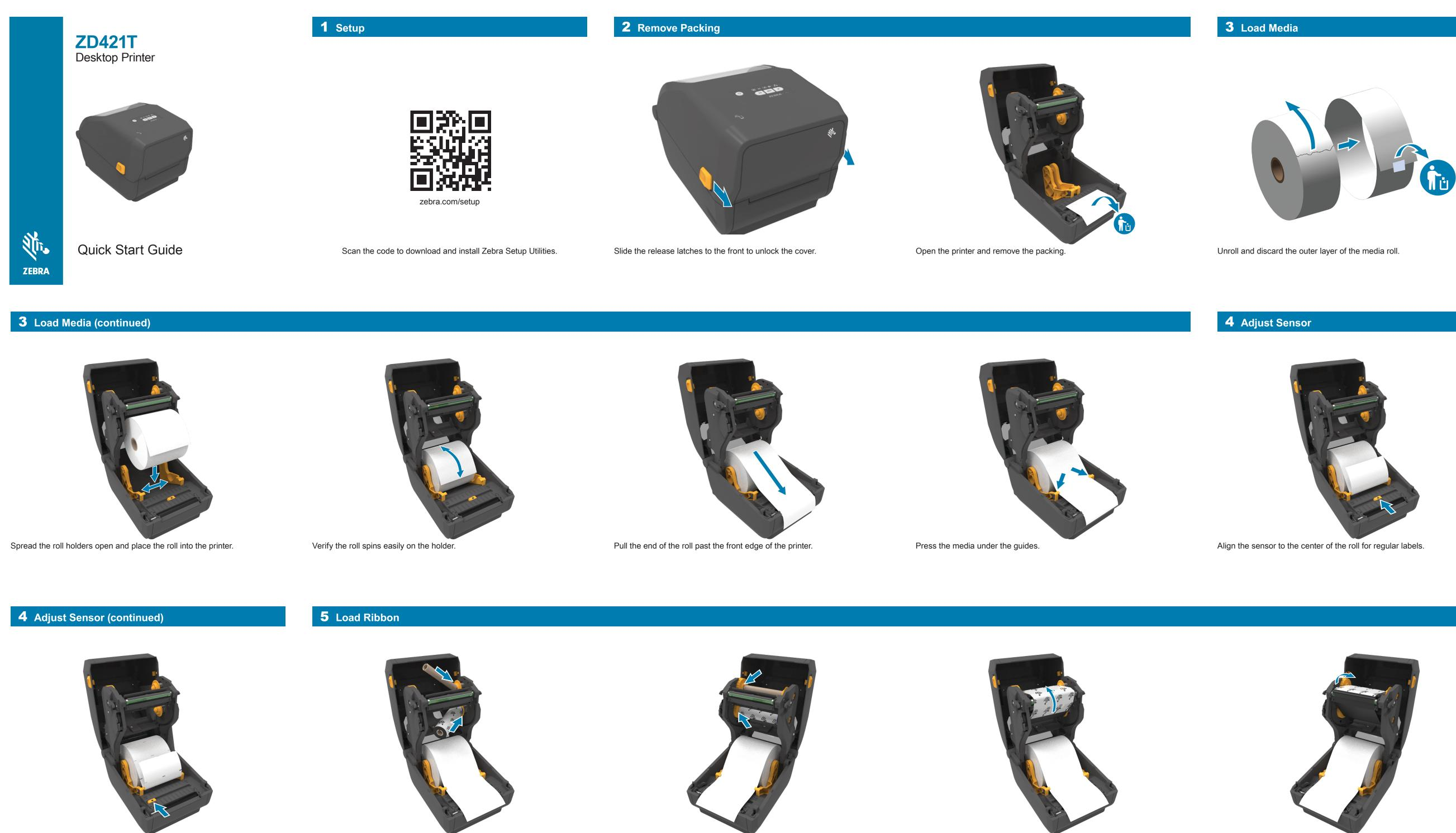
Align the sensor to the edge of the roll for marked labels.
