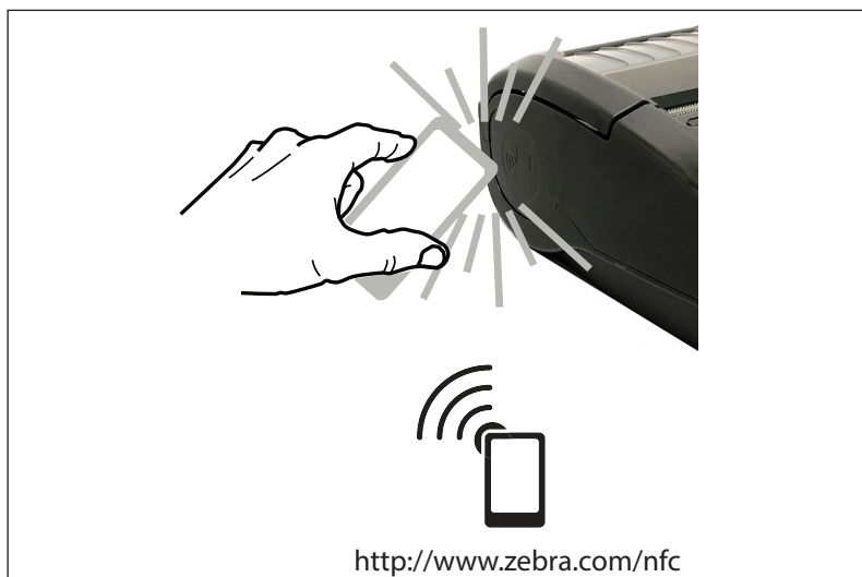
Figure 15 • Near Field Communication (NFC) Pairing
