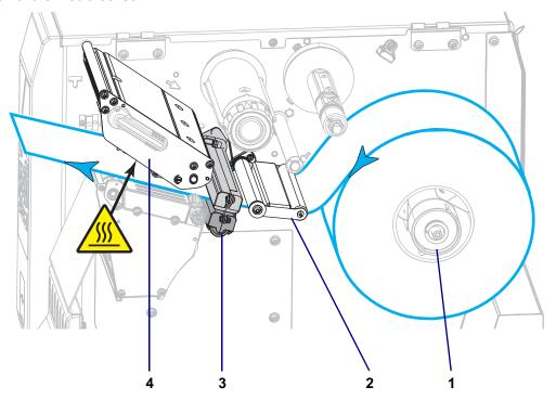
**5.** Rotate the media guide adjustment knob as shown until the media guide just touches the edge of the media.
