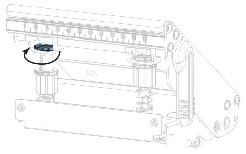
**3.** Reposition the toggle as necessary to provide even pressure on the media. For extremely narrow media, position the inside toggle over the center of the media, and decrease the pressure on the outside toggle.
