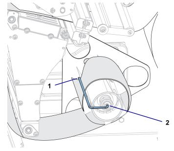
**12.** Rotate the media guide adjustment knob as shown until the media guide just touches the edge of the media.
