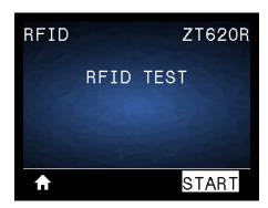
During the RFID test, the printer attempts to read and write to a transponder. No printer movement occurs with this test.
