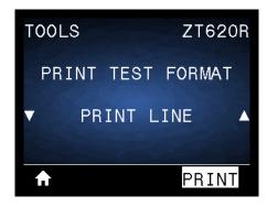
The printer initiates a test sequence that prints an ink/printhead test image multiple times and at varying speeds. These test labels can be used when making adjustments to the printer's mechanical assemblies or to determine if any printhead elements are not working.
