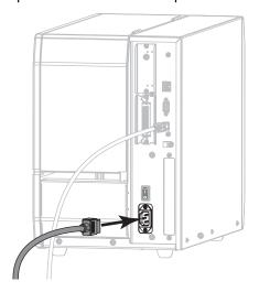
**5.** Plug the male end of the A/C power cord into an appropriate power outlet.
