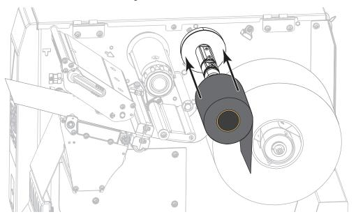
**4.** Bring the ribbon under the printhead assembly and around its left side, as shown.
