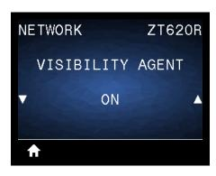
When the printer is connected to a wired or wireless network, it will attempt to connect to Zebra's Asset Visibility Service via the Cloud-based Zebra Printer Connector using an encrypted, certificate-authenticated web socket connection. The printer sends Discovery Data and Settings and Alerts Data. Data printed via any label formats is NOT transmitted.
