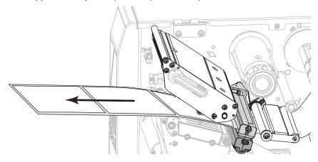
**4.** Remove the exposed labels so that only the liner remains.
