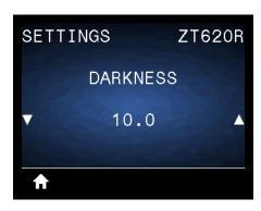
Set the print darkness to the lowest setting that provides good print quality. If you set the darkness too high, the label image may print unclearly, barcodes may not scan correctly, the ribbon may burn through, or the printhead may wear prematurely.
