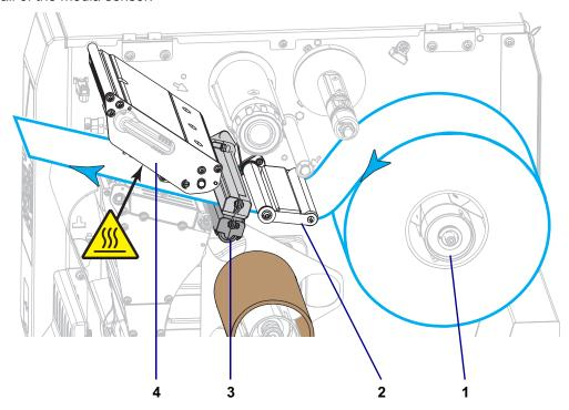
7. Extend approximately 18 in. (500 mm) of media out of the printer.
