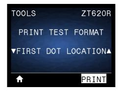
The printer prints an image to assist you with adjusting the position of the image on your labels, if necessary. The lines on the image print from the label top and left edge to identify what should be the top-left corner of the label.
