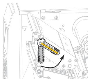
2. Loosen the locking nut at the top of the toggle to be moved.
