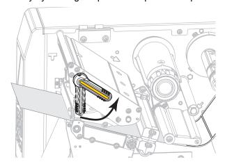
10. Pull the media forward until a label is positioned under the media sensors.
