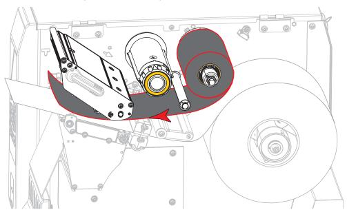
**5.** With the ribbon tracking as far back as it can under the printhead assembly, wrap the ribbon around the ribbon take-up spindle. Rotate the spindle several turns in the direction shown to tighten and align the ribbon.
