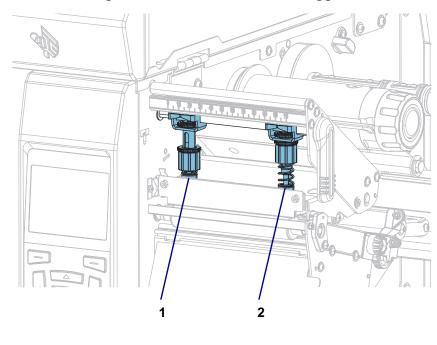
Figure 16 • Printhead Pressure Toggles
