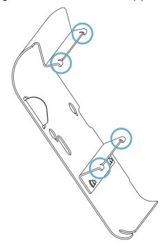
**2-c.** Insert the mounting tabs of the rewind plate into the mounting slots of the printer, and then slide the rewind plate to the left until it will not go any farther.
