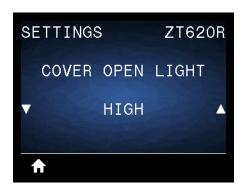
Set the brightness of the light that turns on when the media door is open.
