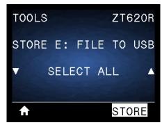
The option **SELECT ALL** is available to store all of the available files from the printer to the USB Flash drive. Any .ZPL file that is copied will be post-processed such that the contents of the file will be suitable to be sent to a printer for normal execution.
