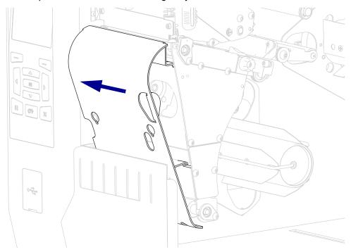
3. Slide a core onto the rewind spindle until it is flush against the guide plate.
