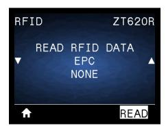
Read and return the specified tag data from the RFID tag located over the RFID antenna. No printer movement occurs while tag data is being read. The printhead can be open or closed.
