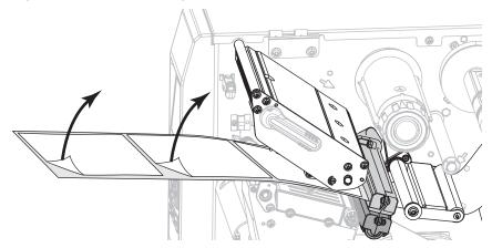
**5.** Pull the media into the printer so that only the backing is over the green light on the lower part of the media sensor.
