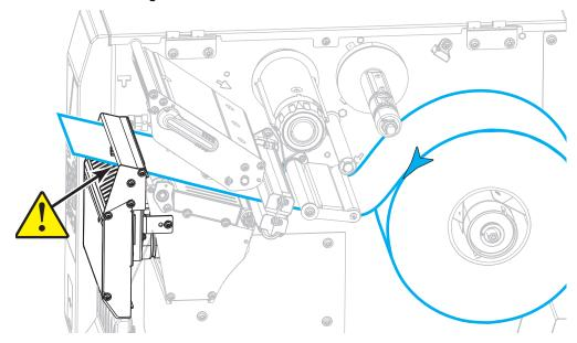
**6.** Rotate the media guide adjustment knob as shown until the media guide just touches the edge of the media.
