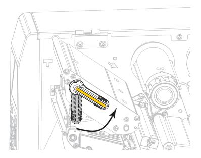
3. Rotate the media guide adjustment knob as shown until the media guide slides all the way out.
