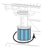
**6.** Hold the lower nut in place and tighten the upper knurled nut.
