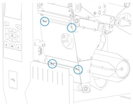
**2-b.** Locate the four mounting tabs on the rewind/liner take-up plate.
