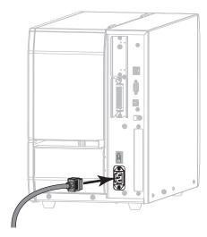
3. Plug the male end of the A/C power cord into an appropriate power outlet.
