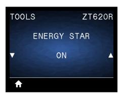
When Energy Star mode is enabled, the printer goes into a "sleep" mode after a timeout period, thereby lowering power consumption. Press any button on the control panel to bring the printer back to an active state.
