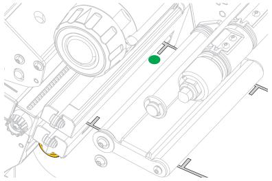
3. If necessary, turn the gold transmissive sensor adjustment wheel to move the sensor until it is positioned at a notch or hole in the media.
