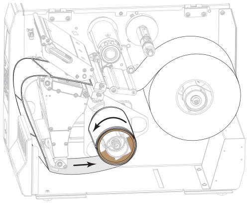
**10.** Rotate the media guide adjustment knob as shown until the media guide just touches the edge of the media.
