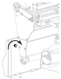
**2-b.** Align the large hole of the keyhole in the rewind/peel plate over the knurled nut, and then slide the plate down until it hits the studs.
