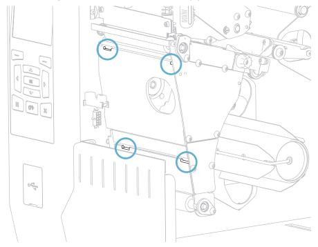
2. Locate the four mounting tabs on the rewind/liner take-up plate.
