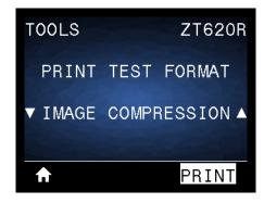
The printer prints an image with diagonal lines, circles, and hash marks at regular intervals around the edges of the image to assist with issues regarding compression or stretching of an image. You can measure the distance between the hash marks or compare the circles and lines to verify if things are being distorted.
