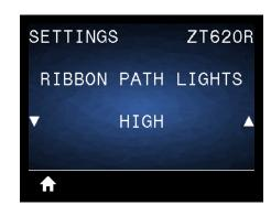
Set the brightness of the lights that illuminate the ribbon path when the ribbon is out.
