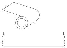
**continuous media** Label or tag-stock media that does not have gaps, holes, notches, or black marks to indicate label separations. The media is one long piece of material wound into a roll. This allows the image to be printed anywhere on the label. Sometimes a cutter is used to cut apart individual labels or receipts.
