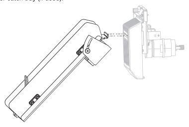
5. Loosen and remove the thumbscrew and lock washer on the cutter shield.
