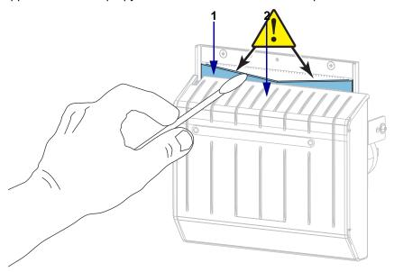
**10.** When the solvent has evaporated, soak a clean swab in a general-purpose, higher-viscosity silicone or PTFE oil lubricant.
