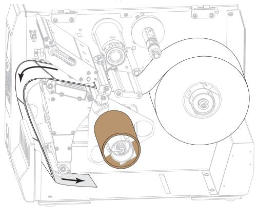
**9.** Wind the media around the rewind spindle as shown. Rotate the rewind spindle several turns to tighten the media and remove any slack.
