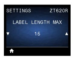
Set a maximum label length that is at least 1.0 in. (25.4 mm) greater than the actual label length plus the interlabel gap. If you set this value too small, the printer assumes that continuous media is loaded and cannot calibrate.
