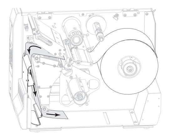
**9.** Remove the hook from the rewind spindle.
