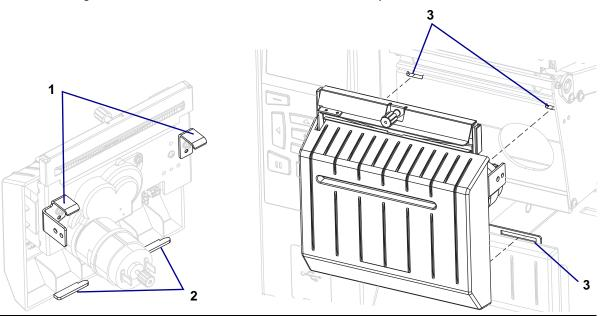
8-f. Slide the cutter module to the left, and then reinstall the cutter mounting screw.
