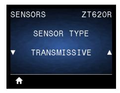
Select the media sensor that is appropriate for the media that you are using. The reflective sensor typically is used only for black mark media. The transmissive sensor typically is used for other media types.
