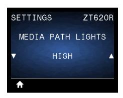
Set the brightness of the lights that illuminate the media path when the media is out.
