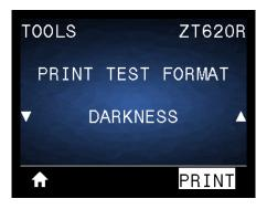
The printer repeats printing an image with incrementing darkness levels. Press CANCEL to stop the printing process at any time when the pattern is clear and legible.
