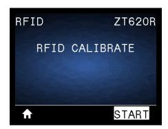
Initiate tag calibration for RFID media. (Not the same as media and ribbon calibration.) During the process, the printer moves the media, calibrates the RFID tag position, and determines the optimal settings for the RFID media being used. These settings include the programming position, the antenna element to use, and the read/write power level to use. See the *RFID Programming Guide 3* for more information.
