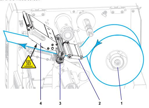
**7.** Extend approximately 18 in. (500 mm) of media out of the printer. Remove and discard the labels from this exposed media, leaving just the liner.
