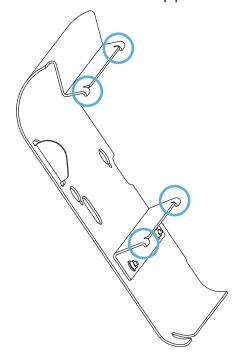
**3.** Insert the mounting tabs of the rewind plate into the mounting slots of the printer, and then slide the rewind plate to the left until it will not go any farther.
