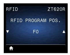
If the desired programming position (read/write position) is not achieved through RFID tag calibration, a value may be specified.
