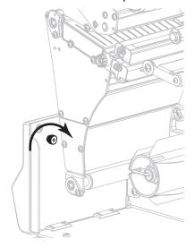
**2.** Align the large hole of the keyhole in the rewind/peel plate over the knurled nut, and then slide the plate down until it hits the studs.
