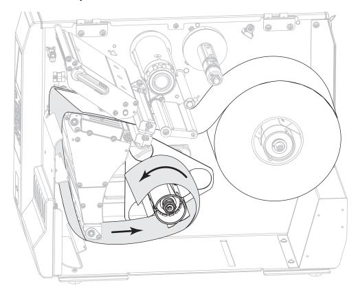
11. Reinstall the spindle hook over the liner. Insert the long end of the hook into the small hole on the guide plate (1). Insert the short end of the hook into the hole in the center of the adjusting nut (2).
