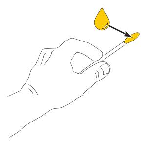
**11.** Apply an even layer along all exposed surfaces of both cutter blades. Remove any excess oil so that none of it comes in contact with the printhead or platen roller.
