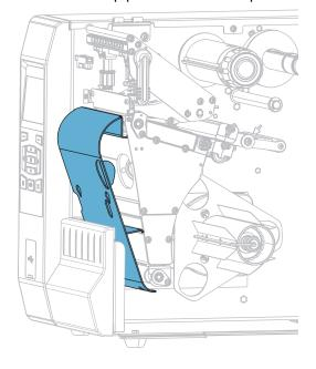
**2-a.** Locate the four mounting slots for the rewind/liner take-up plate.
