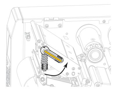
5. Rotate the media guide adjustment knob as shown until the media guide slides all the way out.
