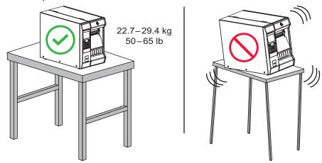
Space: The area where the printer will be located must include enough space for ventilation and for accessing the printer components and connectors. To allow for proper ventilation and cooling, leave open space on all sides of the printer.
