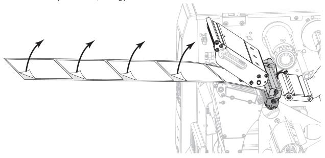
8. Feed the liner behind the rewind/liner take-up plate.
