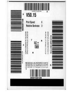
Figure 18 • Sample Darkness and Speed Test Label
