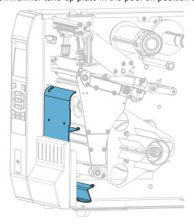
**2-a.** Loosen the knurled nut (1) on the outside stud on the printer's base.
