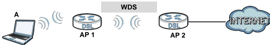
Figure 43 WDS Link Example
