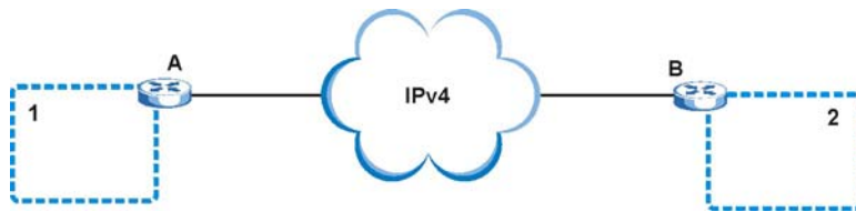
Figure 179 Configured Tunnel Example
