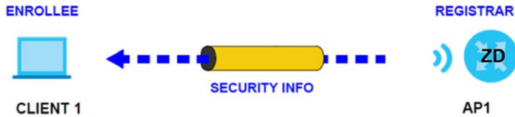
Figure 95 WPS: Example Network Step 1
