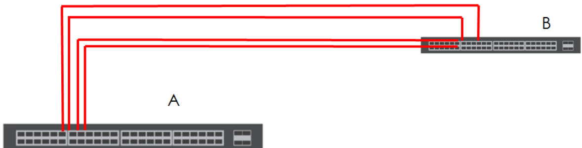
Figure 125 Trunking Example - Physical Connections
