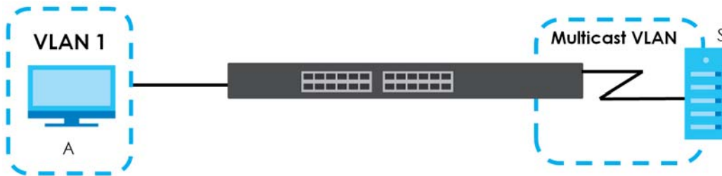
Figure 202 MVR Multicast Television Example
