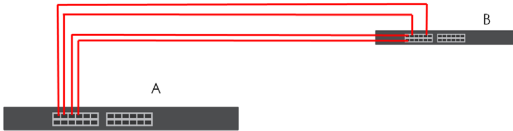
Figure 119 Trunking Example - Physical Connections
