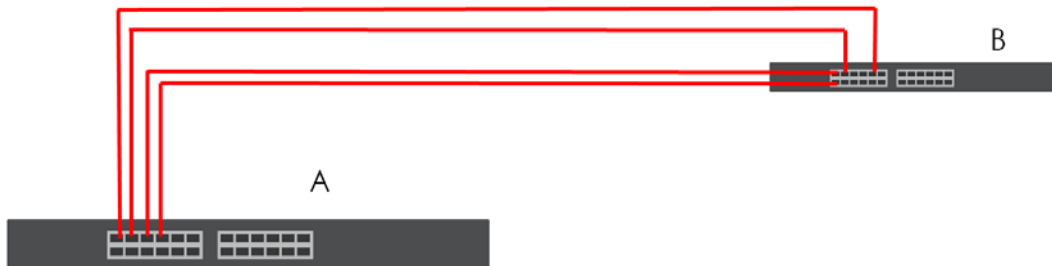
Figure 119 Trunking Example - Physical Connections
